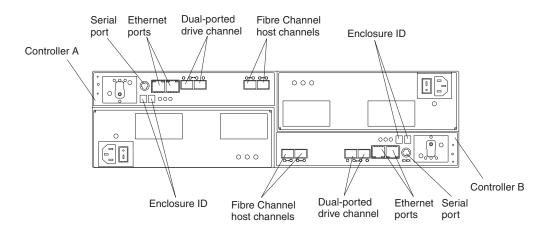
Figure 2. Back view; controllers with two standard Fibre Channel host expansion channels
